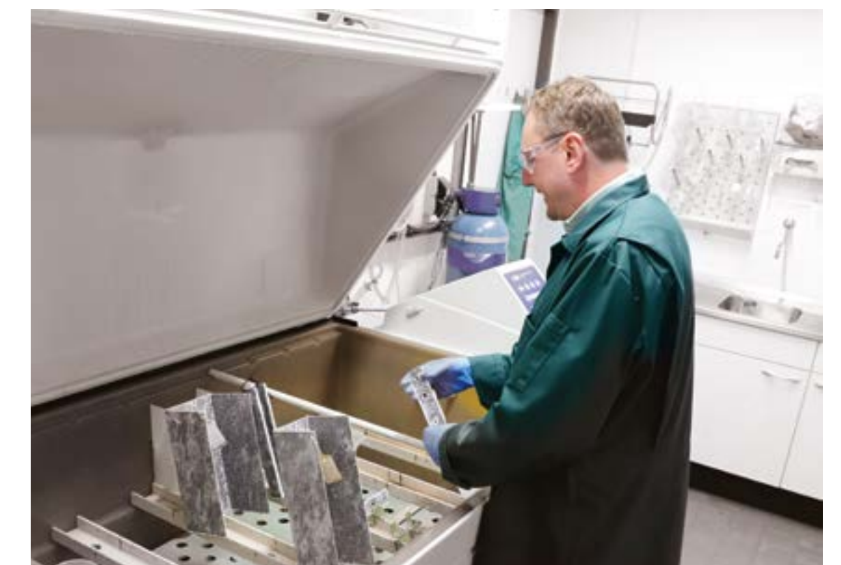
In-house testing (salt spray)
