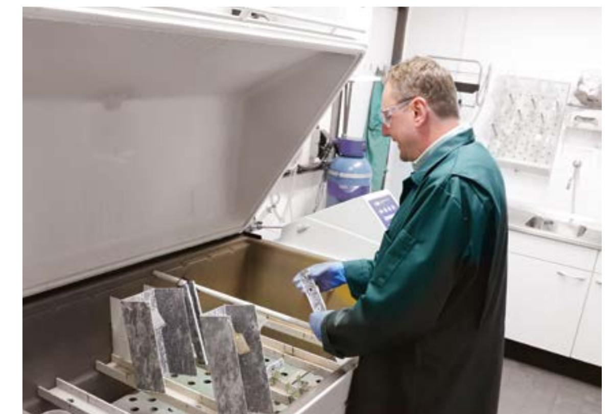
In-house testing (salt spray)
